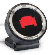
Forward collision warning – receive visual alerts up to 3 seconds before a collision, allowing enough time to react.
